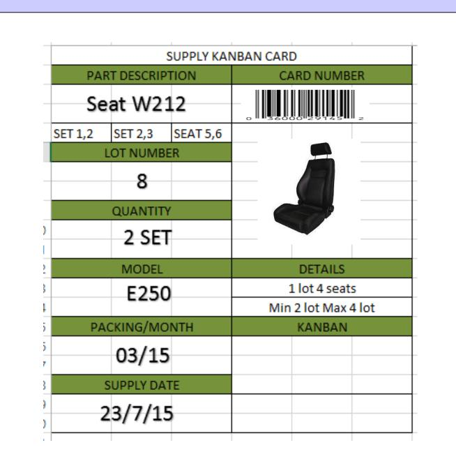
KANBAN CARD AS A TRIGGER FROM CUSTOMER TO THE COMPANY TO RUN THE PRODUCTION.
